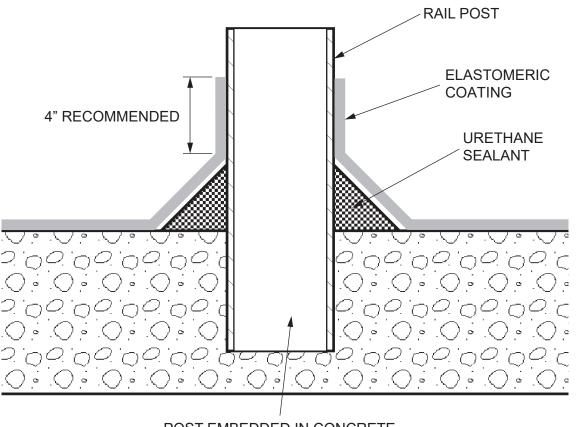
POST EMBEDDED IN CONCRETE OR THREAD-TYPE SLEEVE ANCHORAGE
